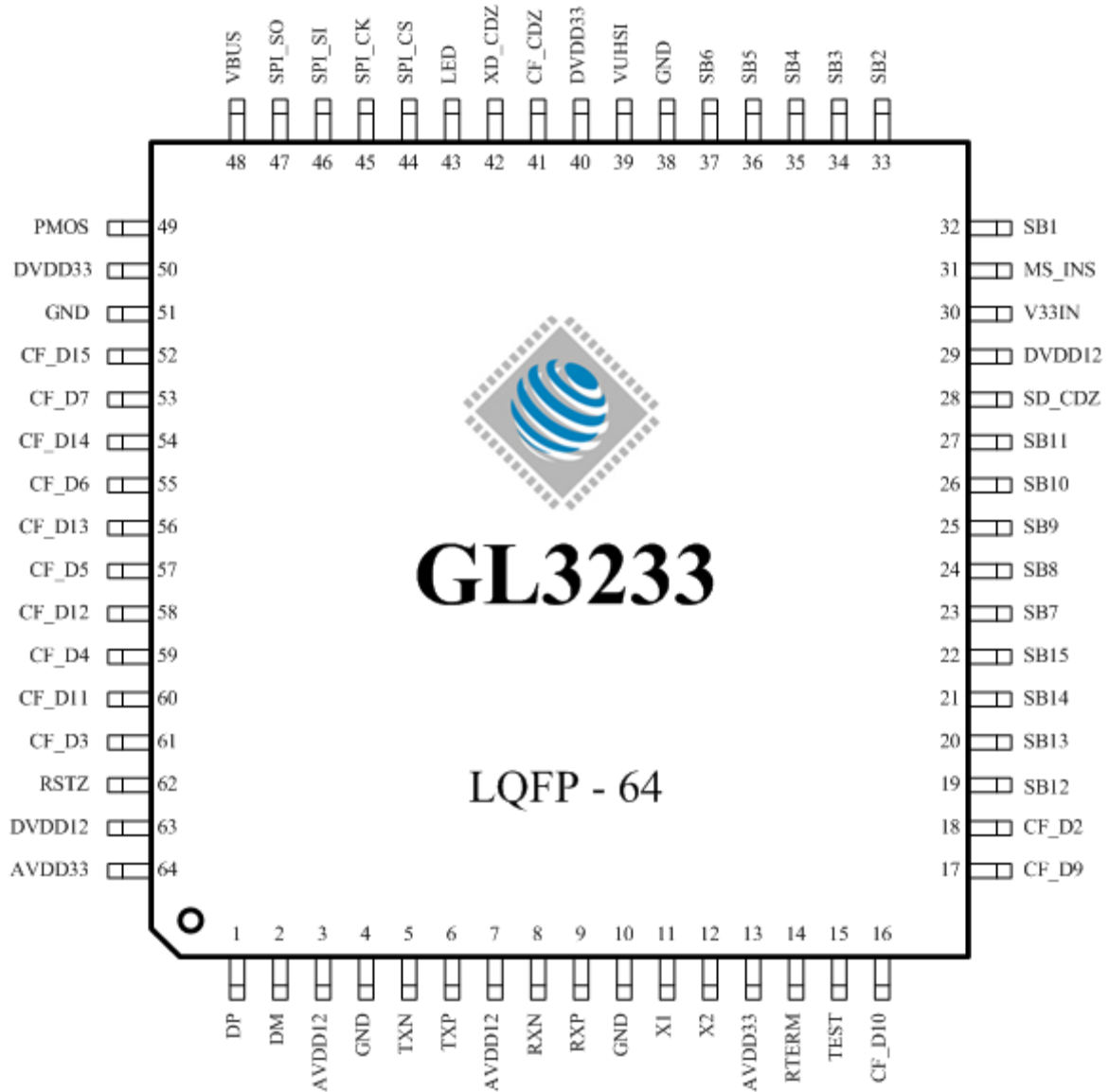
Figure 3.1 - LQFP 64 Pinout Diagram
