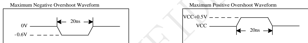
Figure 5-1 Maximum Overshoot Waveform
