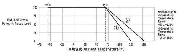
注1: 曲綫①適用于RCMT08產品; 曲綫②適用于RCML08產品。 Note1: RCMT08 product be the same with curve ①; RCML08 be the same with curve ②.
