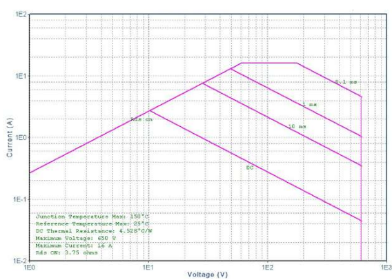
Maximum Safe Operating Area For JCS4N60FB(TO-220MF)
