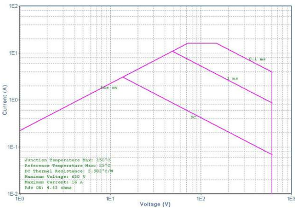
Maximum Safe Operating Area For JCS4N60FB(TO-220MF-K2)
