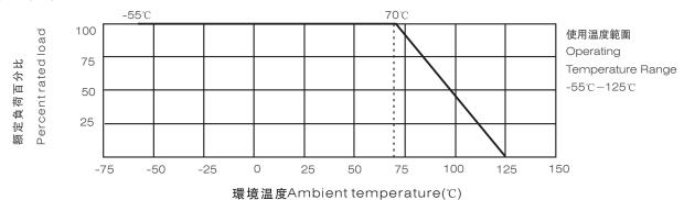
\* 當電阻使用的環境温度超過70℃時,其額定負荷(額定功率或額定電流)按上述曲綫下降。 For resistors operated in ambient over 70°C, rated load (power rating or current rating) shall be derated in accordance with above figure.
