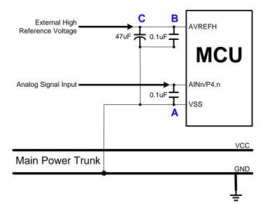
The analog signal is inputted to ADC input pin "AINn/P4.n". The ADC input signal must be through a 0.1uF capacitor "A". The 0.1uF capacitor is set between ADC input pin and VSS pin, and must be on the side of the ADC input pin as possible. Don't connect the capacitor's ground pin to ground plain directly, and must be through VSS pin. The capacitor can reduce the power noise effective coupled with the analog signal.
