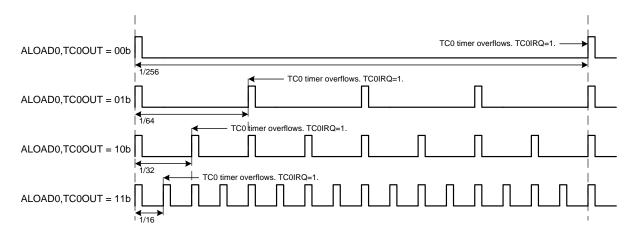
The PWM output pin is shared with GPIO and switch to output PWM signal as PWM0OUT=1 automatically. If PWM0OUT bit is cleared to disable PWM, the output pin exchanges to last GPIO mode automatically. It easily to implement carry signal on/off operation, not to control TC0ENB bit.
