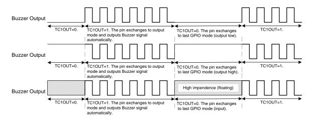
Example: Setup TC10UT output from TC1 to TC10UT (P5.3). The external high-speed clock Fhosc is 4MHz. the instruction cycle Fcpu is Fhosc/4. The TC10UT frequency is 0.5KHz. Because the TC10UT signal is divided by 2, set the TC1 clock to 1KHz. The TC1 clock source is from external oscillator clock. TC1 rate is Fcpu/8. The TC1RATE2~TC1RATE1 = 101. TC1C = TC1R = 131.
