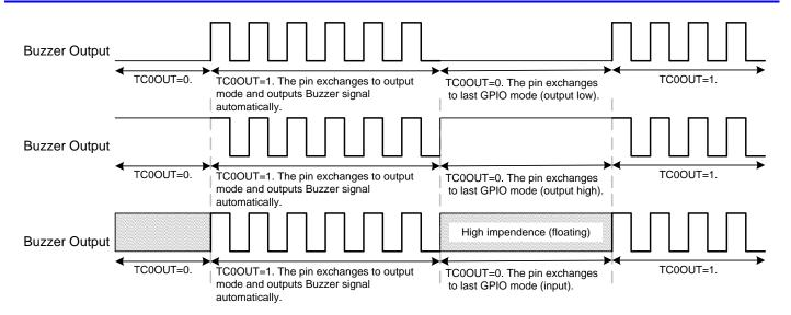
Example: Setup TC0OUT output from TC0 to TC0OUT (P5.4). The external high-speed clock Fhosc is 4MHz. the instruction cycle Fcpu is Fhosc/4. The TC0OUT frequency is 0.5KHz. Because the TC0OUT signal is divided by 2, set the TC0 clock to 1KHz. The TC0 clock source is from external oscillator clock. TC0 rate is Fcpu/8. The TC0RATE2~TC0RATE1 = 101. TC0C = TC0R = 131.
