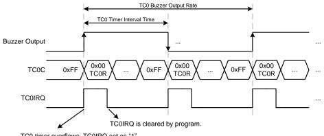
TC0 timer overflows. TC0IRQ set as "1". Reload TC0C from TC0R automatically.
