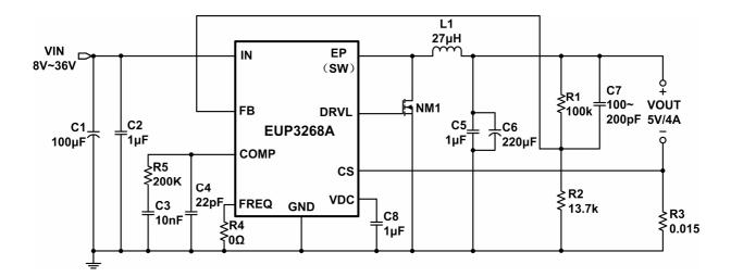
Figure 1. Application Circuit
