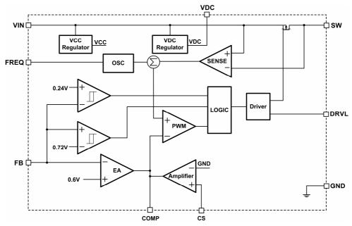
Figure 2. Functional Block Diagram
