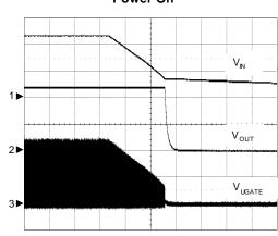
CH1:  $V_{\rm IN}$ , 5V/Div CH2:  $V_{\rm OUT}$ , 500mV/Div CH3:  $V_{\rm UGATE}$ , 10V/Div Time: 200ms/Div
