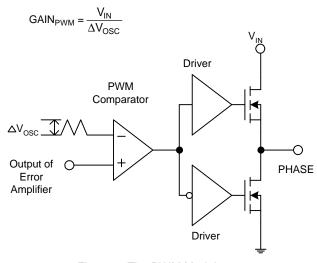
Figure 4. The PWM Modulator
