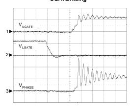
$\begin{array}{l} \text{CH1: V}_{\text{UGATE}}, 20\text{V/Div} \\ \text{CH2: V}_{\text{LGATE}}, 10\text{V/Div} \\ \text{CH3: V}_{\text{PHASE}}, 10\text{V/Div} \\ \text{Time: 20ns/Div} \end{array}$
