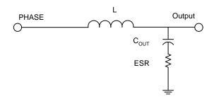
Figure 2. The Output LC Filter
