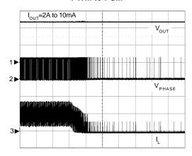
CH1:  $V_{OUT}$ , 500mV/Div CH2:  $V_{PHASE}$ , 10V/Div CH3:  $I_L$ , 2A/Div Time: 500 $\mu$ s/Div
