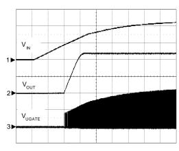
CH1:  $V_{\rm IN}$ , 5V/Div CH2:  $V_{\rm OUT}$ , 500mV/Div CH3:  $V_{\rm UGATE}$ , 10V/Div Time: 1ms/Div
