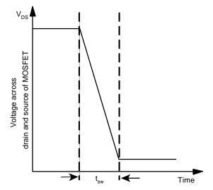
Figure 7. Switching waveform across MOSFET
