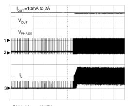
CH1:  $V_{OUT}$ , 1V/DivCH2:  $V_{PHASE}$ , 10V/DivCH3:  $I_L$ , 2A/DivTime:  $500\mu s/Div$
