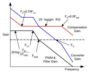
Figure 6. Converter Gain & Frequency
