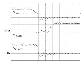
CH1: V<sub>UGATE</sub>, 20V/Div CH2: V<sub>LGATE</sub>, 10V/Div CH3: V<sub>PHASE</sub>, 10V/Div Time: 20ns/Div
