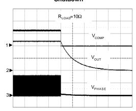
CH1: V<sub>COMP</sub>, 1V/Div CH2: V<sub>OUT</sub>, 500mV/Div CH3: V<sub>PHASE</sub>, 10V/Div Time: 1ms/Div
