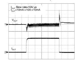
CH1:  $V_{OUT}$ , 50mV/Div CH2:  $I_{OUT}$ , 5A/Div Time: 100 $\mu$ s/Div
