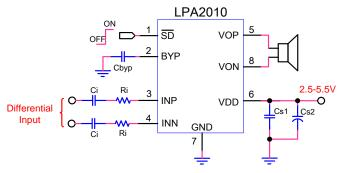
LPA2010 Application Schematic With Differential Input
