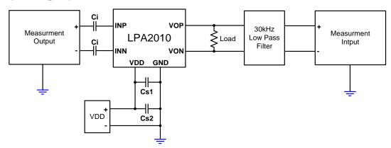
1. Ci was shorted for any common-mode input voltage measurement. All other measurements were taken with CI = 0.1µF (unless otherwise noted).
