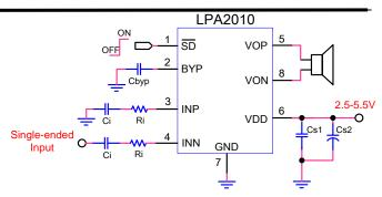
LPA2010 Application Schematic With Single-Ended Input
