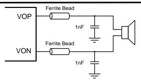
Typical ferrite-bead output filter
