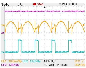
V<sub>IN</sub>=12V, V<sub>OUT</sub>=3.3V, I<sub>OUT</sub> =2.0A
