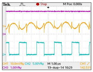
$V_{IN}$ =9V,  $V_{OUT}$ =3.3V,  $I_{OUT}$  =2.0A
