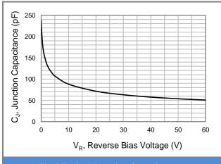
Fig.5 Typical Junction Capacitance
