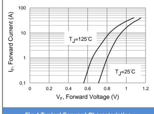
Fig.4 Typical Forward Characteristics
