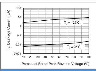
Fig.3 Typical Reverse Characteristics
