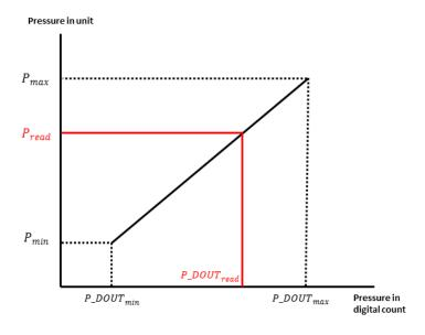
For example, the  $P_{min}$  and  $P_{max}$  for the sensor are specified as -0.1 and +0.1 psi. The  $DOUT_{min}$  and  $DOUT_{max}$  are -26214 and +26214. So,
