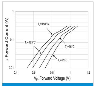
**Fig.1 Typical Forward Characteristics**
