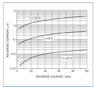
FIG. 2 TYPICAL REVERSE CHARACTERISTICS
