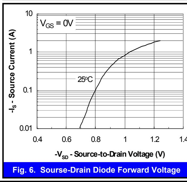
Fig. 6. Source-Drain Diode Forward Voltage
