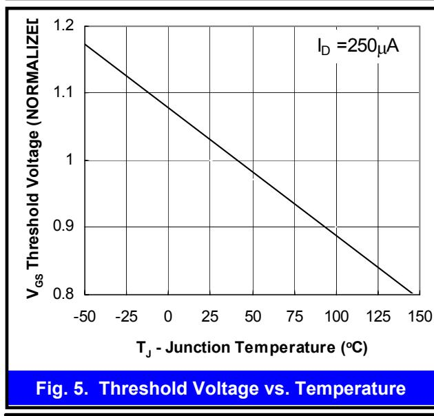
Fig. 5. Threshold Voltage vs. Temperature
