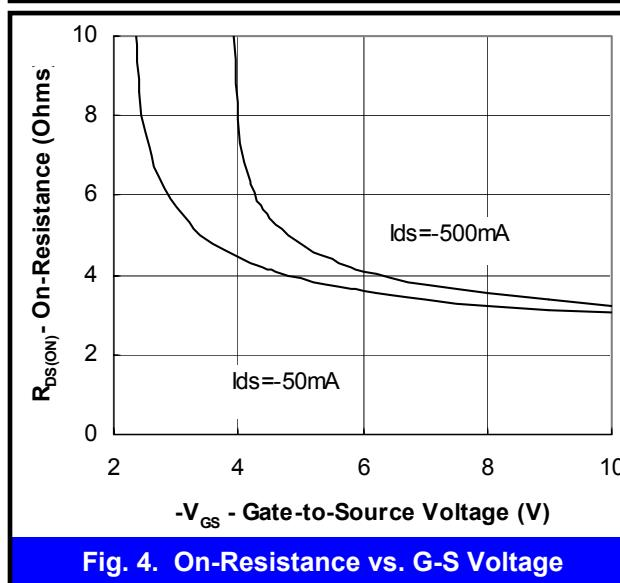
Fig. 4. On-Resistance vs. G-S Voltage
