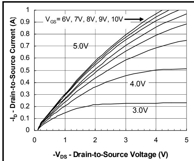
Fig. 1. Output Characteristics
