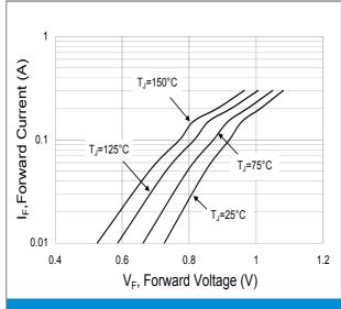
Fig.%Typical Forward Characteristics
