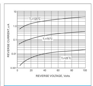
FIG. 2 TYPICAL REVERSE CHARACTERISTICS
