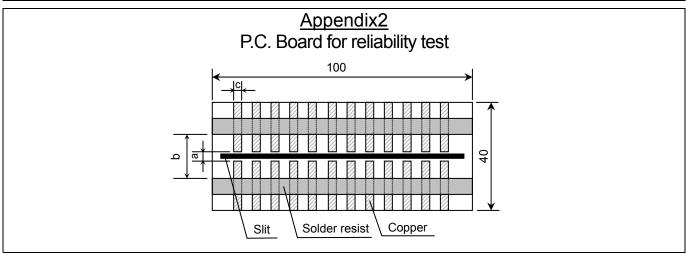
(It is recommended to provide a slit on P.C. board for CGA6,CGA8 and CGA9.)
