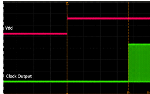
Figure 16. Startup Waveform vs. Vdd
