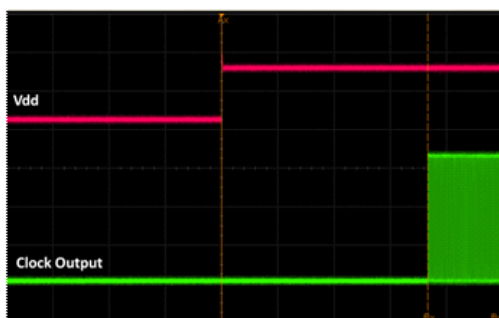
Figure 17. Startup Waveform vs. Vdd
