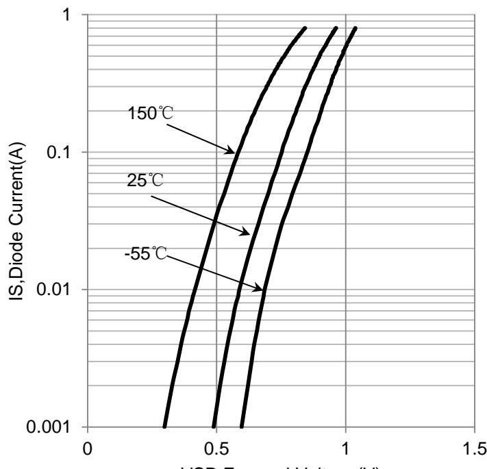
Body Diode Forward Voltage
