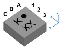
**Note:** Coordinates shown above indicate polarity after a SET operation.
