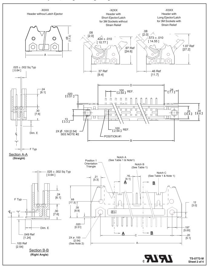
.100" × .100" Latch/Ejector, Straight and Right Angle
