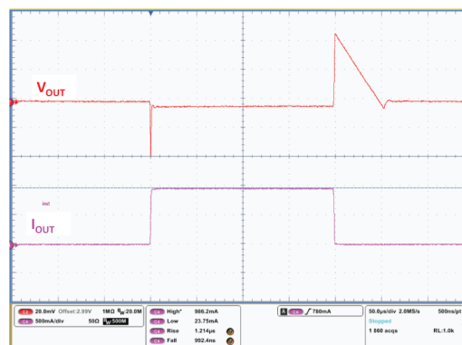
Figure 24. Load transient ( V_{IN} = V_{EN} = 3.5\text{ V} ; t_{RISE} = 1\text{ µs} ; I_{OUT} = 1\text{ mA} to 1\text{ A} )
