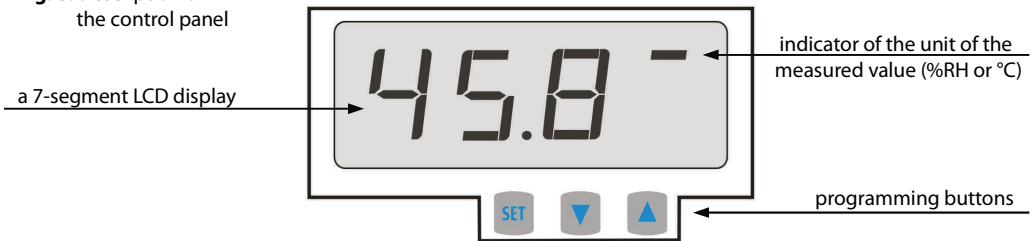
Fig. 8. Description of the control panel
