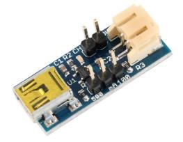
This small circuit can recharge in an extremely simple way Li-Po and Li-Ion cells. Using a jumper with two positions you can select two possible values for the charging current, 100mA and 500mA; the correct value should be chosen in consultation with the characteristics of the battery.
