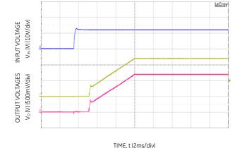
Figure 1. Typical Start-up Using On/Off Voltage ( $V_{IN} = 12V$ ,  $I_0 = I_{O1,max}$ ,  $I_{O2,max}$ ).
