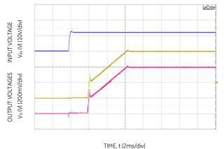
Figure 5. Typical Start-up Using On/Off Voltage (Vin=12V, Io = Io1,max, Io2,max,).
