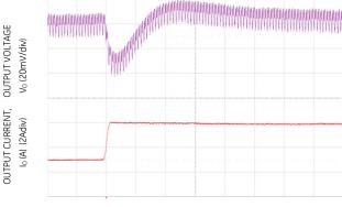
Figure 15. Typical output ripple and noise (Co= 2×4.7nF+2×47uF ceramic, Vin = 12V, Io = Io1,max, Io2,max).
