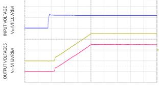
Figure 35. Typical Start-up Using On/Off Voltage ( $V_{IN} = 12V$ ,  $I_{O} = I_{O1,max}$ ,  $I_{O2,max}$ ).
