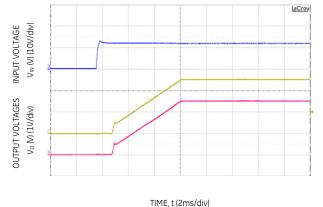
Figure 23. Typical Start-up Using On/Off Voltage ( $V_{IN} = 12V$ ,  $I_0 = I_{01,max}$ ,  $I_{02,max}$ ).
