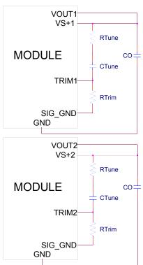
Figure. 47. Circuit diagram showing connection of  $R_{\text{TUNE}}$  and  $C_{\text{TUNE}}$  to tune the control loop of the module.
