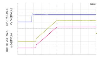
Figure 29. Typical Start-up Using On/Off Voltage (V<sub>IN</sub> = 12V, I<sub>o</sub> = I<sub>o1,max</sub>, I<sub>o2,max</sub>).
