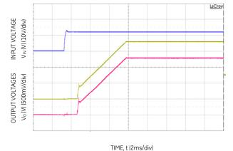
Figure 17. Typical Start-up Using On/Off Voltage ( $V_{IN} = 12V$ ,  $I_0 = I_{01,max}$ ,  $I_{02,max}$ ).
