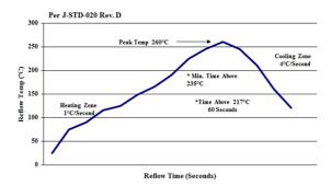
Figure 51. Recommended linear reflow profile using Sn/Ag/Cu solder.
