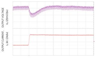
Figure 9. Typical output ripple and noise ( $C_0$ = 2×4.7nF+2×47uF ceramic,  $V_{IN}$  = 12V,  $I_0$  =  $I_{01,max}$ ,  $I_{02,max}$ ).
