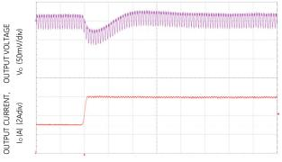
Figure 21. Typical output ripple and noise ( $C_0$ = 2x4.7nF+2x47uF ceramic,  $V_{IN}$  = 12V,  $I_0$  =  $I_{01,max}$ ,  $I_{02,max}$ ).
