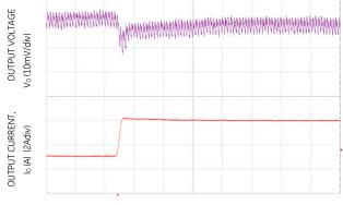
Figure 3. Typical output ripple and noise ( $C_0$ = 2×4.7nF+2×47uF ceramic,  $V_{IN}$  = 12V,  $I_0$  =  $I_{01,max}$ ,  $I_{02,max}$ ).
