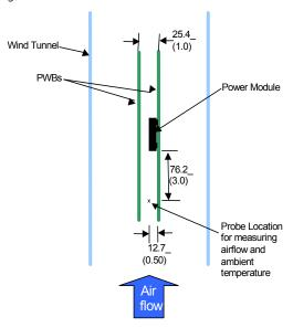
Figure 49. Thermal Test Setup.
