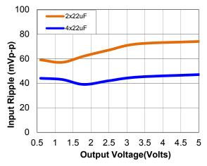
Figure 37. Input ripple voltage for various output voltages with 2x22 µF or 4x22 µF ceramic capacitors at the input (2 x 6A load). Input voltage is 12V. Scope BW: 20MHz
