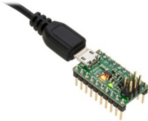
A-Star 32U4 Micro with soldered headers and connected USB cable.
