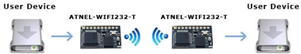
Figure 26. Transparent Serial Port Application
