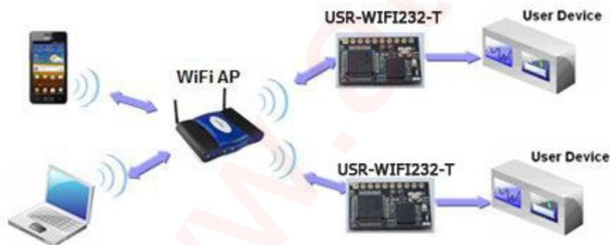
Figure 6. ATNEL-WIFI232-T Basic Wireless Network Structure.
