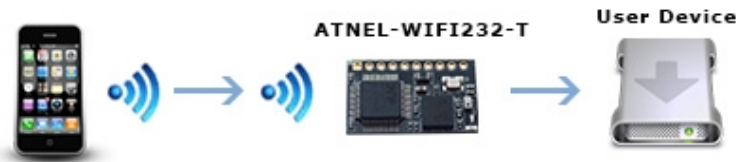
Figure 24. Wireless Control Application
