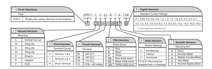
Note: Terminals 1 & 2 are standard for current ratings  $\leq$  12A Terminals 2 & 3 are standard for current ratings > 12A Terminals 1, 2 & 3 are optional for current ratings  $\leq$  6A
