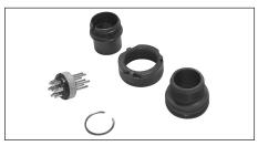
Unassembled connectors are supplied in kits, an insulator kit and hardware kit. The insulator kit includes a snap ring and insulator with preloaded contacts. The hardware kit includes the shell along with appropriate endbell (except box mount receptacles) and coupling nut (plug only).
