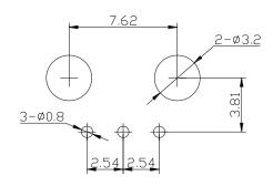
Note: General Tolerance :±0.2mm, Substrate Thickness:1.6mm, Unit = mm
