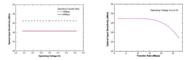
Note: Before using the EAPLRBA2 device, please confirm the minimum sensitivity at different operating voltage and transmission rate.
