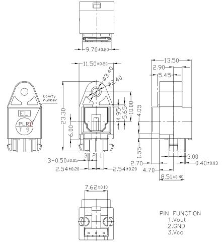
Note: Tolerances unless mentioned ±0.3mm. Unit = mm
