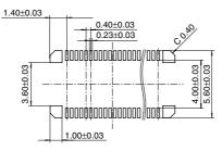
Recommended metal mask pattern Metal mask thickness: When 150  $\mu$ m (Terminal portion opening area ratio: 53%) (Metal portion opening area ratio: 100%)
