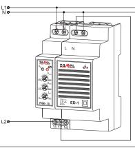
Control and L1 phase voltage drop signalling circuit.
