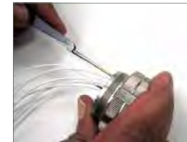
Removal of contacts with metal tool.
