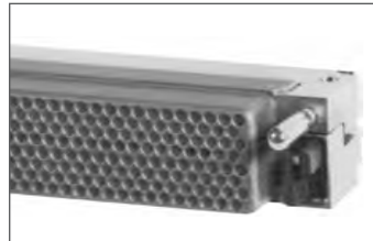
GEN-X Grid - Up to 472 Contacts in 8 Rows.
