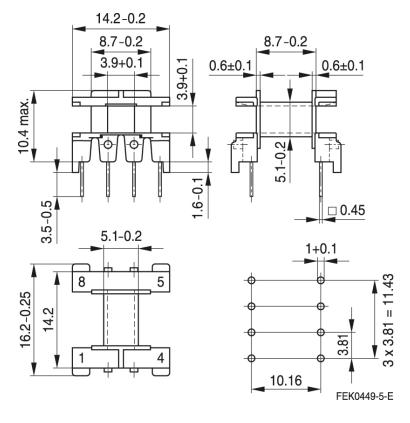
Hole arrangement View in mounting direction
