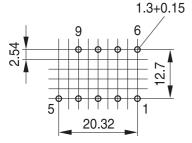
Hole arrangement View in mounting direction
