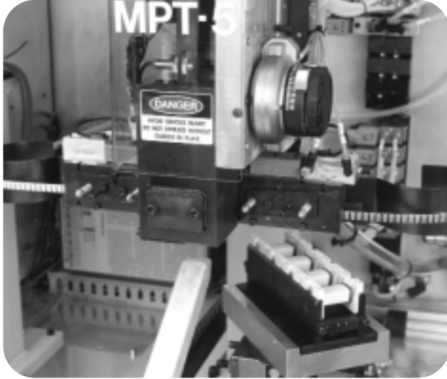
Rotary Index Insertion Process
