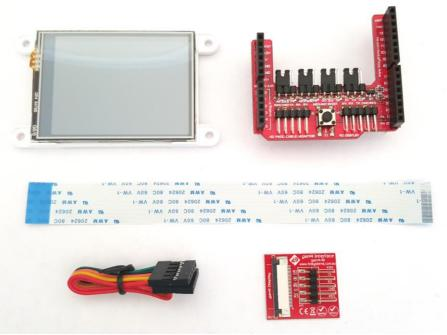
Components in a typical gen4 AR Kit.
