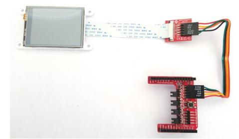
Components in the AR Kit connected together. Arduino Adaptor Shield shown then connects on top of the customers Arduino board (not included).
