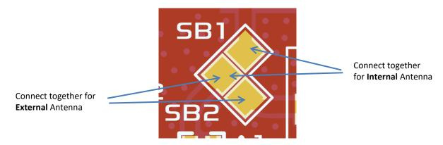
**Note:** If both SB1 and SB2 are connected at the same time, then WiFi performance may be impacted, as both the internal and the external antenna will be enabled at the same time.
