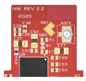
By default, SB1 is soldered closed with a solder blob, which enables the ESP32 to be connected to the internal antenna on the rear side of the PCB.
