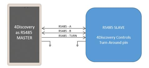
This image shows the 4Discovery when acting as Master, connecting to a Slaved device which is incapable of Auto turn-around, but can have its RS485 chip controlled externally by the 4Discovery. Not a typical situation.
