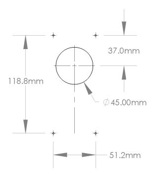
The 4 corner holes are actually slots on the plastic, which give some tolerance when mounting. The slots actually allow for 51.15mm to 56.15mm horizontal centres.
