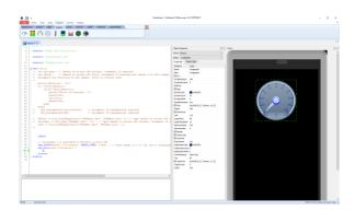
Workshop4 PRO adds a professional set of features to the ViSi environment, called Smart Widgets. These smart widgets allow Users to create custom gauges, sliders, buttons and more, rather than relying on the built-in ones. This provides an extra level of customisation available for intelligent products.
