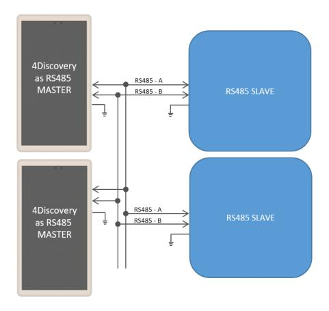
**Figure 4.** This shows multiple Masters on the RS485 network, with multiple Slaves. A specialised program and protocol is required to realise this setup, but is useful if more than one 4Discovery is required on the network to control the same set of equipment from multiple locations.
