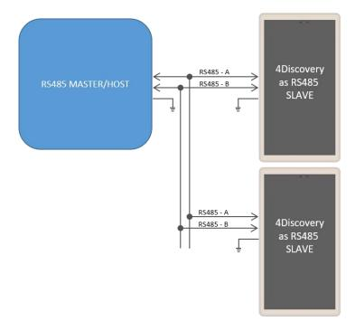
**Figure 3.** This shows the situation where there are 1 or more Slaves on the network, of which 1 or more could be a 4Discovery. Each Slave needs to handle the changing of its own Transmit/Receive, based on the information received from the Master. Only one Slave should reply at any given time, after the Master has transmitted to it. Utilizing RS485 transceivers with Auto Direction control can simplify the setup, however a suitable protocol needs to be utilized regardless.
