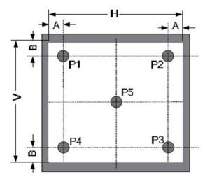
Figure 3. The definition of viewing angle
