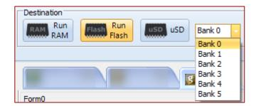
The additional drop-down menu allows the user to specify the target destination flash bank of the ViSi-Genie program. The Diablo16 processor has six flash banks (Bank 0 to Bank 5), each of which has a capacity of 32 kB.
