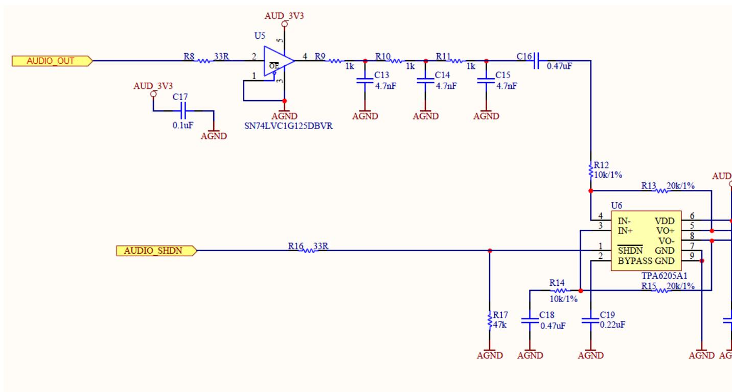
Please note this circuit is not included on any hardware from 4D Systems. This is a reference schematic from FTDI, which can be used to filter and amplify audio signals coming from the FT800, and therefore 4DLCD-FT843 Display.
