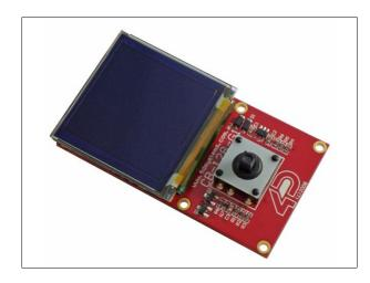
The **CB-128-G1** is a compact carrier board designed to provide a simple means of adding user input to the already capable uOLED-128-G1(SGC) (Serial Platform) and the uOLED-128-G1(GFX) (4DGL Platform) range of intelligent display modules. The tiny 5-position joystick, along with an on-board speaker, facilitates user input and output for these displays.
