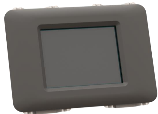
gen4-uLCD-24DT Mounted in 2.4" Bezel - Front
