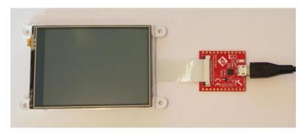
Figure 1. Typical connection of gen4 display module to gen4-PA with USB cable (not included)
