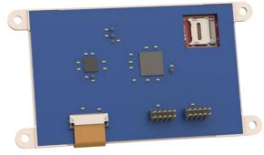
The 30 way FFC flex cable out of the gen4 into the application board can either turn up through a slot in the application board, or can travel down under the gen4 plastic and emerge at the bottom, and then into the application board (as depicted above).
