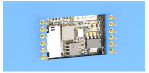
The IoD-09SM features surface mount castellated pads, and is designed to be soldered in place onto a host PCB. This module can be mounted on a PCB in 2 main ways.
