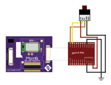
• While GPIO 9 of the gen4 PA is grounded, connect the GPIO10 (Reset) pin to Ground for a second and disconnect it (Reset) from Ground.
