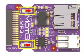
Unless the designer intends to use two UART MOTGs on a gen4-MOTG-AC2 or gen4-MOTG-AC4 board, the UART pins should be directed to TX, RX of the UMI as shown above.
