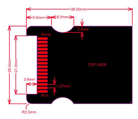
The MOTG boards are designed in such a way that the leading edge (header end) of the MOTG modules is a fixed design, and depending how complex the MOTG module is, will determine how long the board itself is. By default, the standard MOTG module is around 38mm in length, but can be extended longer if required. Note that depending on the target application, longer boards may have mounting challenges.
