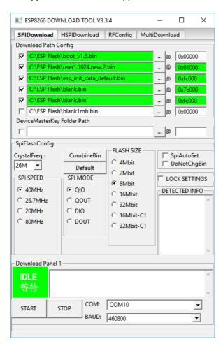
It will be noticed there are six different files preloaded into the Download Path Config boxes. These need to be changed to the location where the files were extracted to.
