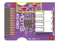
Unless the designer intends to use two UART MOTGs on a gen4-MOTG-AC2 or gen4-MOTG-AC4 board, the UART pins should be directed to TX, RX of the UMI as shown above.
