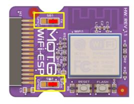
Unless the designer intends to use two UART MOTGs on a gen4-MOTG-AC2 or gen4-MOTG-AC4 board, the UART pins should be directed to TX, RX of the UMI as shown above.
