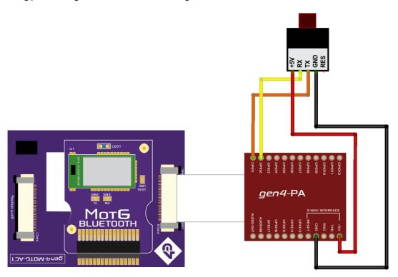
The RN4870 needs to be placed into Test mode. The following procedure will place the Bluetooth module in Test mode.
