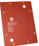
Where the Application PCB is shown to sit in Section 5.5, can house a small metal shield of the same size. This shield is used instead of, or underneath an Application PCB, to aid the on-board electronics in the prevention from potential RF or EMI signals.
