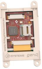
The image below (2.4" model depicted) shows a mock Application PCB on the back of the gen4 display (Blue area). It features a cut-out in the PCB so access to the micro-SD socket on the gen4's display board is possible, however this may or may not be required depending on the application and if the micro-SD socket is utilised or requiring access once the Application PCB is applied.
