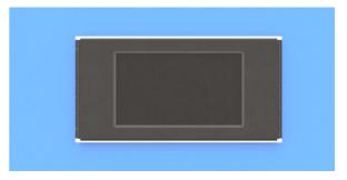
A hole the size of the rear of the module, with enough clearance for the electronics, be formed in the product, and the IoD-SM sits in the hold with the surface mount pads being soldered from the front, and its electronics accessed through the hole.
